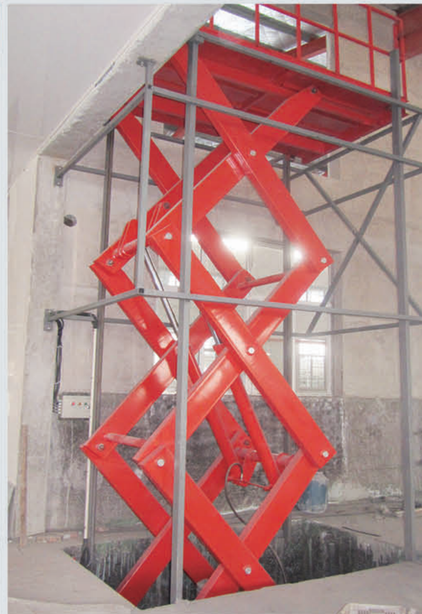
Scissor lift for carrying cargos from ground to the first floor
