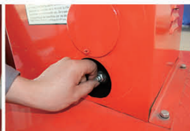
Emergency drop valve
