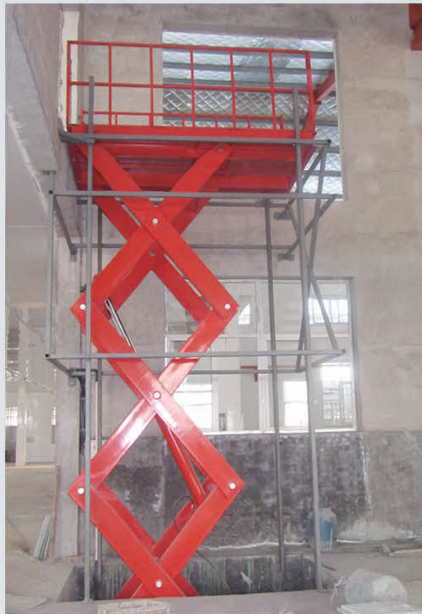
Scissor lift for carrying cargos from ground to the first floor
